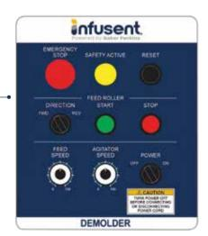
Simple start/stop pushbuttons, a speed potentiometer, a safety switch, and emergency stop button provide safety and an easy-to-use controls system.
