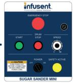
The operator controls consist of simple Start/Stop pushbuttons and a Speed potentiometer. Additionally, a safety system is incorporated to monitor the removable guards and the Emergency Stop
